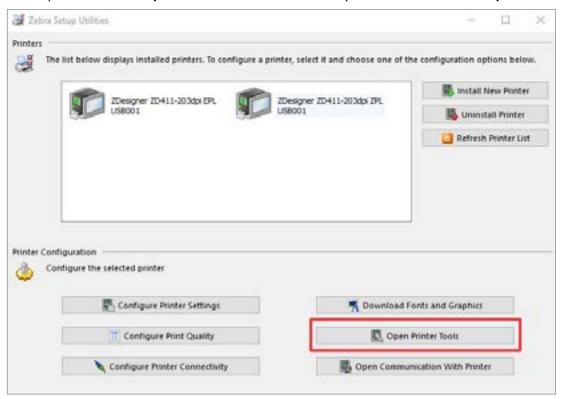
This can also be done from Devices and Printers > right-click > Printer Properties > click on the Driver Settings tab.
