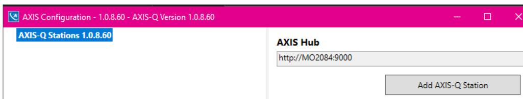
3. In the **AXIS Hub** field, highlight the URL and **copy the path** (right-click > Copy or Ctrl+C).
